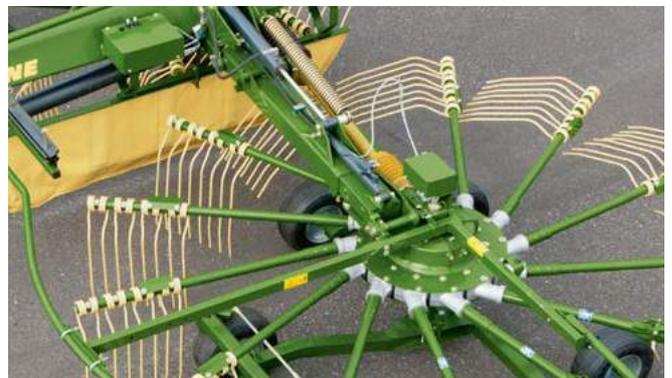
**The rotor suspension system\***
