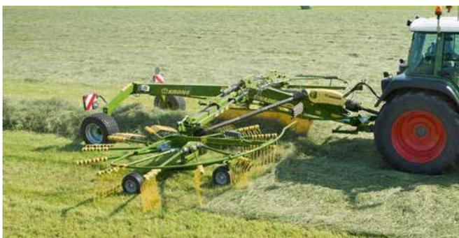
Swadro TS 970 triple-rotor side delivery rake
