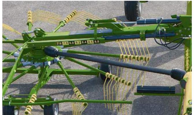
**Changing work widths hydraulically**
