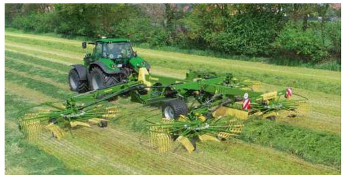
Swadro 1400 and 1400 Plus four-rotor centre delivery rakes
