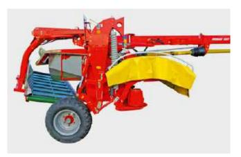
When driving over mowed crop, you need a lifting system that is convenient to use and provides a generous lifting height.
