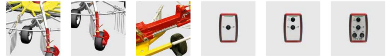
**Jockey wheel inside rotor arc**      **MULTITAST jockey wheel**      **Hydraulic working width adjustment**      **Individual hydraulic lift system**      **Individual hydraulic lift system incl. transport interlock**      **Hydraulic height adjustment**
