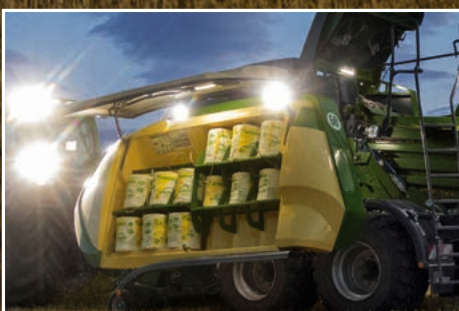
Lights inside the twine boxes
