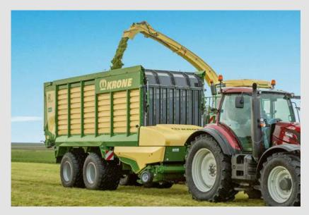
The MX 330 GL/GD as forager-filled wagon Its rugged steel structure and the high 18t axle load make the MX 330 the most reliable and productive companion for the forage harvester.
