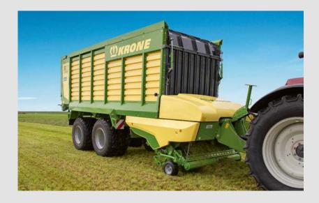
The MX 330 GL/GD as self-loading wagon Fast and consistent fills are key and attributed to the wide work width of the pick-up and the rotor cutter as well as the wide and short feed chamber. Blades with wavy edges and plated rotor tines ensure a particularly high quality of cut.
