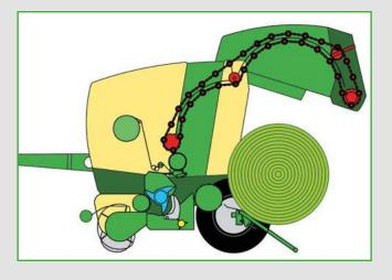
and so the baling cycle finishes earlier as well. The elevator also creates a firmer core and packs more weight and density into each bale, which translates into higher quality silage and better exploitation of truck capacities.
